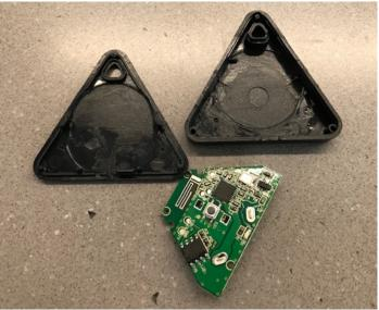
Simple twist function securing compartment – can be opened by hand:
