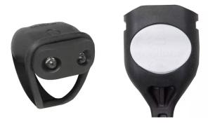
Fobs and remote controls that are designed to have a coin as 'tool'. Often can be pushed open by hand, or do not meet drop test requirements:
